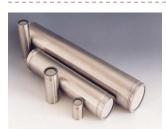
Nal(TI) crystal is a kind of scintillation crystal with good properties. It is grown by host material sodium iodide doped with appropriate percentage of thallium. Its emission maximum is 415nm, which is well matched to the sensitivity curve of photomultiplier tubes (PMTs) with bialkali
