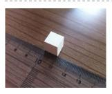
CsI(TI) crystal emission maximum is 550nm, which is well matched to the sensitivity curve of photomultiplier tubes (PMTs) with bialkali photocathodes. CsI(TI) crystal is relatively soft, can be made into a variety of shapes, able to withstand the mechanical and thermal shock.
