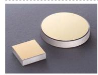
Total reflection mirrors coated with gold (Au) that has high reflectance in a wide range of infrared. Chromium (Cr) is slightly undercoated to reinforce adhesion of gold to the substrate. Gold mirrors of silicon substrates have higher durability than glass substrates because gold coating adheres to silicon much stronger and silicon substrate has higher thermal conductivity.
