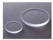
Used as transparent barriers for sending and receiving light between two phases under varying conditions in temperature, pressure, chemical composition, cleanliness, and phase. Windows of synthetic optical MgF2 are highly abrasion-resistant, with hardness approaching that of diamonds. The material allows transmission of light in the range from ultraviolet to near-infrared.
