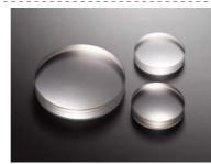
Achromatic doublets are cemented by two kinds of lenses, low dispersion positive (crown glass) and high dispersion negative (flint glass). The differences of dispersions and shapes of both lenses are designed to minimize the chromatic aberrations at blue (486.1nm), green
