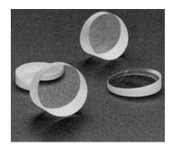
Wedge prism is an optical element with plane-inclined surfaces, usually the faces are inclined toward one another at a very small angles. It diverts light toward its thicker portion. Wedge prisms can be used as isolating components. Wedges may also be used to produce a small deviation which doesn't allow return to source.
