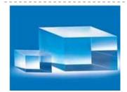
Rhomboid prisms are used to displace a laser beam without changing its direction. In imaging applications, they will displace the optical centerline without inverting the image. The lateral displacement is equal to the length of the prism ("D" dimension). High tolerance angles
