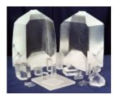
Potassium Dihydrogen Phosphate (KDP) and Potassium Dideuterium Phosphate (DKDP or KD\*P) are among the most widely-used commercial NLO materials, characterized by good UV transmission, high damage threshold, and high birefringence, though their NLO coefficients are
